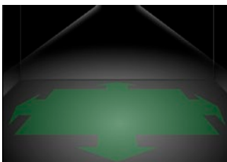
Escape route illumination with symmetric optics
