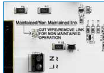
Configurable as Maintained or Non-Maintained operation
